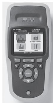
Figura 4.2 - Analisador Wireless Professional Fluke.
